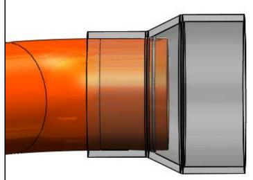
12. Once you have installed both silicone boots over each of the CAC tubes. You can now install the PAS valve. Please note the flow orientation arrow on the side of the casting. This is the direction of air flow.
