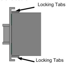
5. Change the position selection switch to position #2 (Auto Test). Slide enclosure cover over circuit board.
