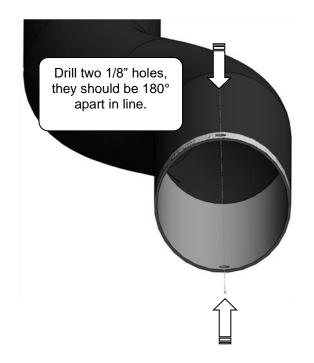
8. Once the pilot holes are drilled you will need to drill an Ø11/32" hole through the pilot holes.
