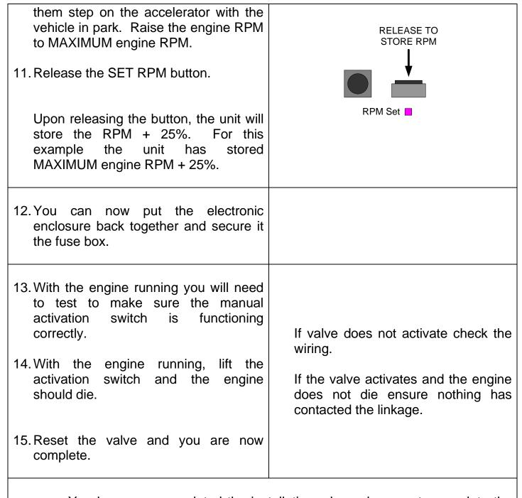
You have now completed the installation, please be sure to complete the test once a year to make sure the unit is functioning correctly.
