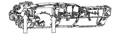
Using a 1/8" drill, drill a pilot hole in the location you have selected for the switch to be mounted.
