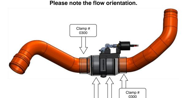
13. Install all clamps loosely until proper in-vehicle fitment can be determined.
