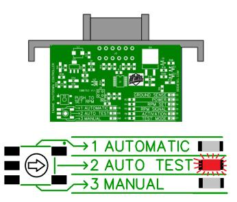
6. Start the vehicle, with the vehicle in park step on the throttle increasing the engine RPM. At 1200RPM the PAS should engage itself automatically, and the engine should stall. Like with all activations the toggle switch should flash.
