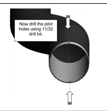
9. Once the holes are drilled, install the ring bead around the pipe. Lock each end of the ring bead into each hole.
