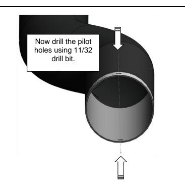
Once the holes are drilled, install the ring bead around the pipe. Lock each end of the ring bead into each hole.
