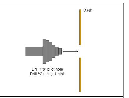
18. Once you have the mounting hole drilled, crimp the switch connectors to the switch wires and install the correct switch wires to the correct switch terminals, then insert the switch into the dash from the backside.
