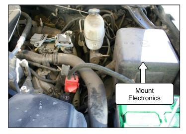
30. Double check all wiring connections and ensure wires are routed away from any heat sources and moving parts. And continue to the Setup, Testing and Verification with Over Speed Electronics section in this manual.
